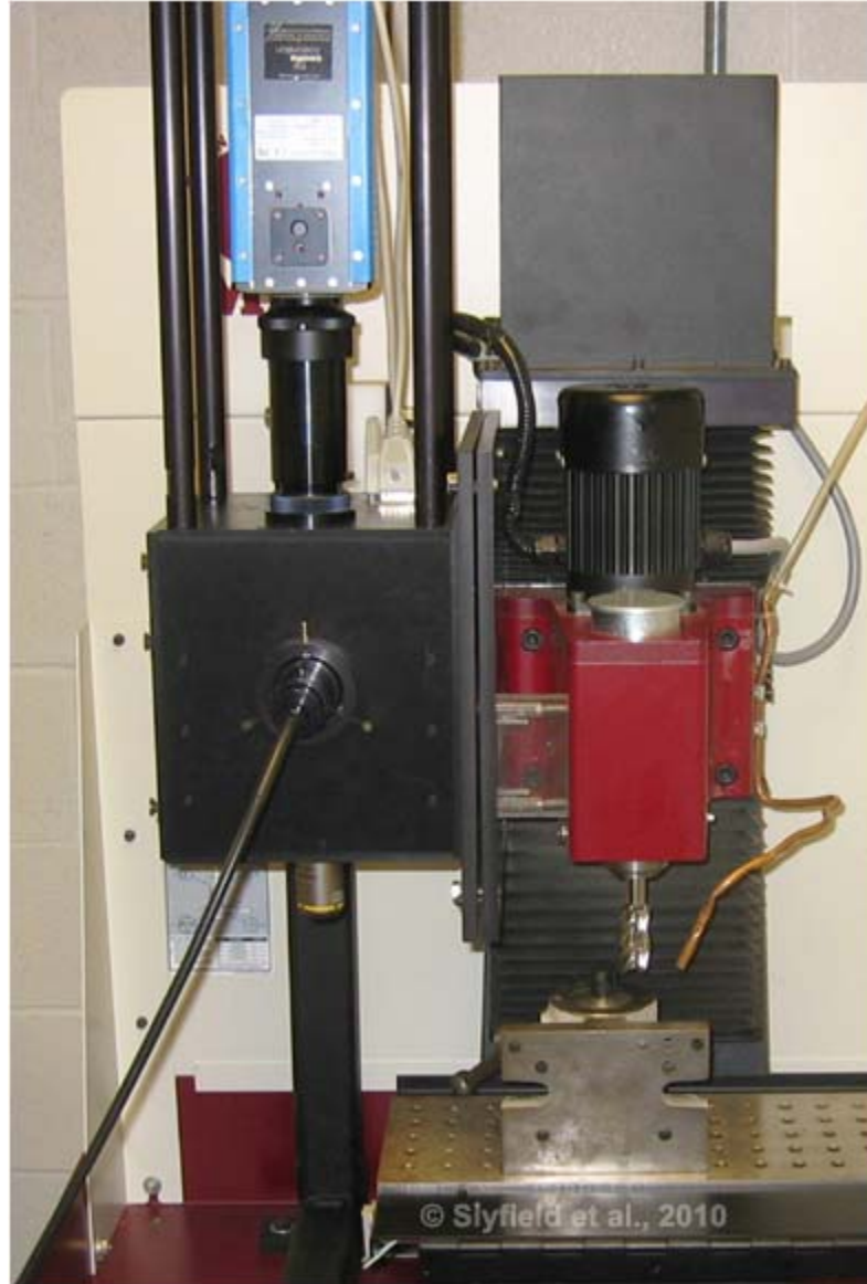
Figure 4-1. Serial fluorescence microscopy is accomplished using a CNC milling device. An attached grayscale camera, automated filterset changer, and microscope objective lens are used to serially and automatically acquire images of each cross-section.
